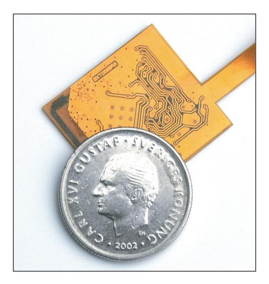
Senscon provides the worlds smallest cellular phone integrated IEEE 802.15.4 compatible sensor node. SensCoin™ integrates Your sensors with your favourite cellular phone.The solution is here - What is Your application?
