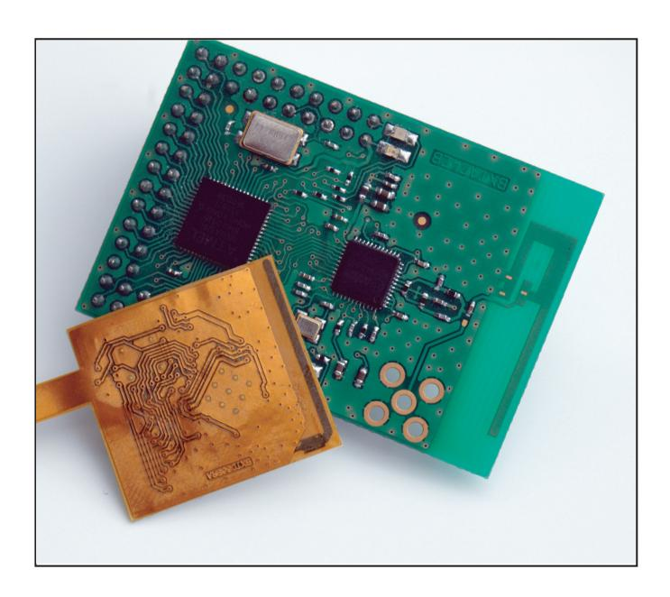
Senson provides a flexible sensor network environment based on IEEE 802.15.4 compatible sensor nodes. Modules for product integration as well as modules for integration in cellular handsets. are available.
